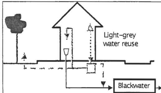
These systems are usually closed systems that collect greywater from shower and bathroom basin within an underground tank where the water is disinfected using continuous UV before re-use for toilet flushing and external garden watering. Storage tank volumes need to be optimised depending on the reuse intention.
